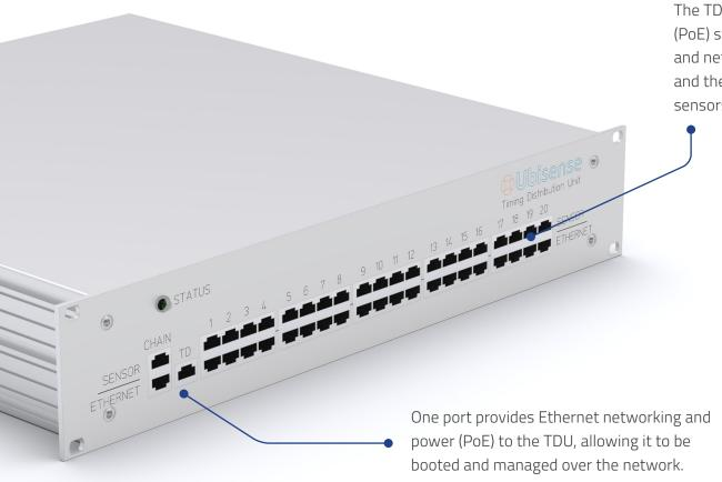
The TDU has 21 ports to be connected to a Power-over-Ethernet (PoE) switch as well as 21 ports to be connected to sensors. Power and networking are passed onto these ports from the PoE switch, and the TDU injects an additional timing signal used by Ubisense sensors onto unused signal lines in the cable.
