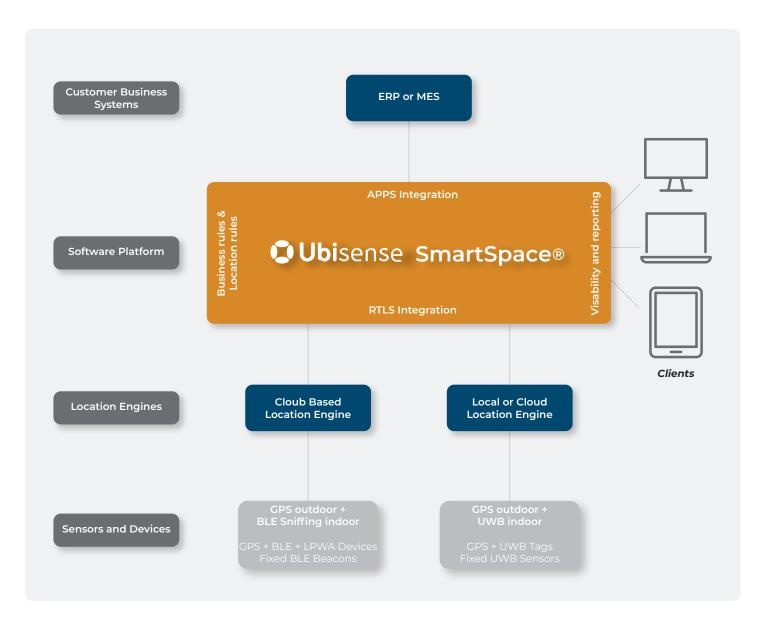
Ubisense SmartSpace takes any location sensor data, including Ultra-Wideband, Bluetooth Low-Energy and GPS, and integrates with existing tooling, maintenance and calibration systems to provide insight and control via any browser-enabled device.
